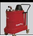
same time. Emptying is as easy as flipping a switch. Our pump removes liquids at 38 gallons per minute, and the vacuum features an 8" discharge plate for solid matter. The compression cast composite housing will never dent or rust. The float assembly monitors liquid intake thus, eliminating the chance for overflow.
