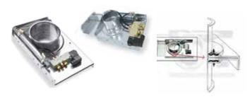
Truly "air-tight" blast gates operate manually or pneumatically and utilize a two part, self-sealing gasket assembly to completely isolate outside air, guaranteeing no air leakage across the valve or into the atmosphere. Designed to withstand 16 Hg" of negative pressure. Available in Zinc Plate or Stainless Steel.
